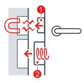
The magnetic movement latch creates new silence standard when the door closes.
