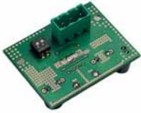
Amplifier card 30 W, 24 V dc for 6-8 Ohm impedance speakers
