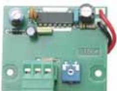
Amplifier card 8 W, 24 V dc, for 8 Ohm impedance speakers
